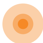
ORANGE MULTIMODE OM1 62.5/125 \mu\text{m}
