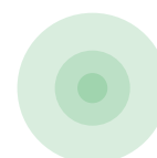
LIME GREEN MULTIMODE OM5 50/125 \mu\text{m}
