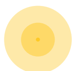
YELLOW MONOMODE G652D OR G657A2 9/125 \mu\text{m}
