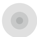
GREY MULTIMODE OM2 50/125 \mu\text{m}
